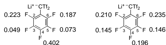
Figure 2. Frontier electron densities (left) and atomic charges (right) of the NLUMO at C2–C5 in the lithium salt of 2 .
